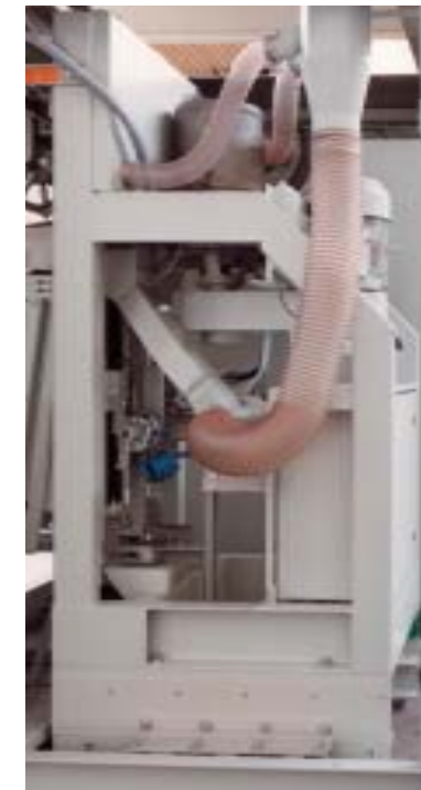
Horizontal impeller filling system
