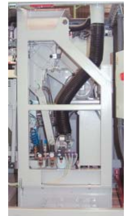
Vertical impeller filling system
