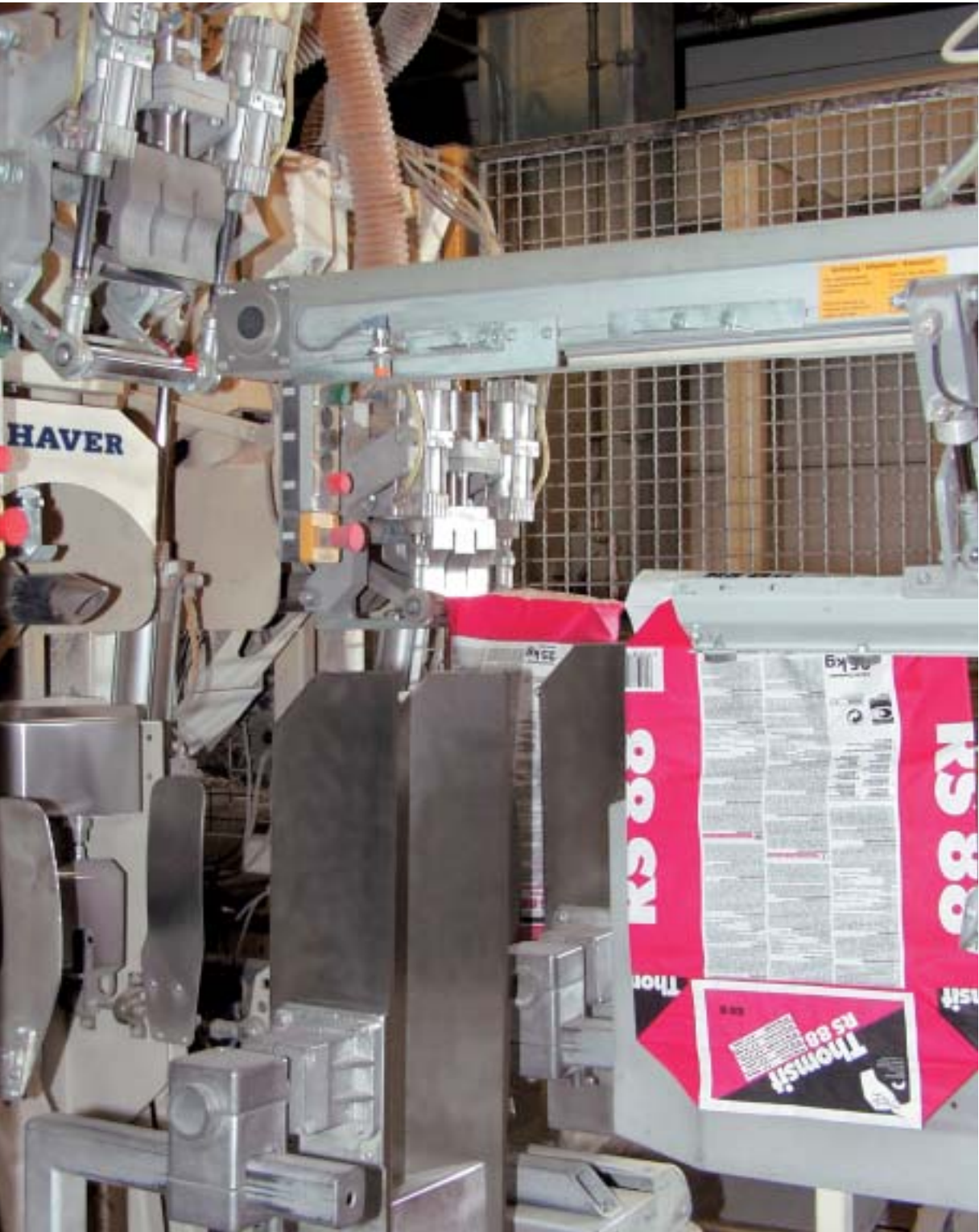
Fully automatic HAYER valve-bag filling machine with valve closing and automatic bag applicator
