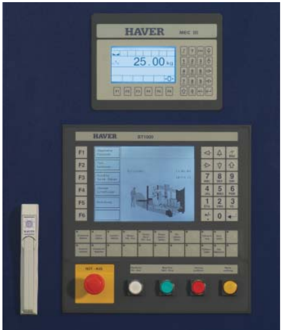
Top picture: FFS operator interface with weigher terminal and MEC III and operator panel BT1000.
