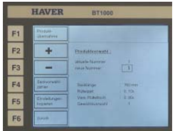
Right picture: Operator panel DT1000 with product pre-select function.
