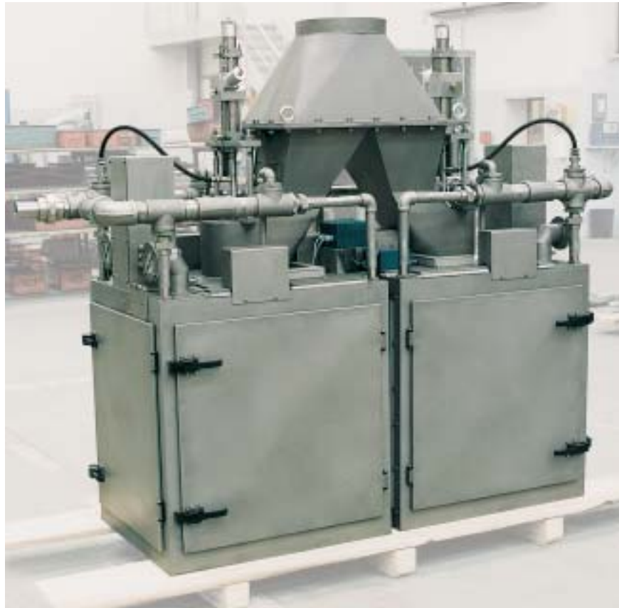
Top picture: Duplex weigher with automatic water wash down.
