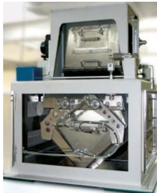
Top picture: Duplex weigher with automatic water wash down.
